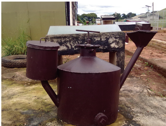
Fig. 2. 136L Capacity Metallic Prototype Biodigester
