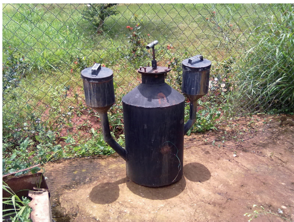
Fig. 1. 50L Capacity Metallic Prototype Biodigester
