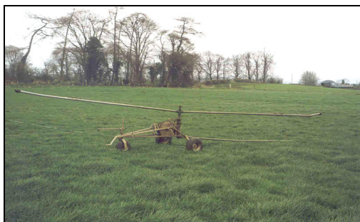
Photo 2. Rotational centre pivot sprinkler system used for dairy dirty water irrigation (Source: www.teagasc.ie )
